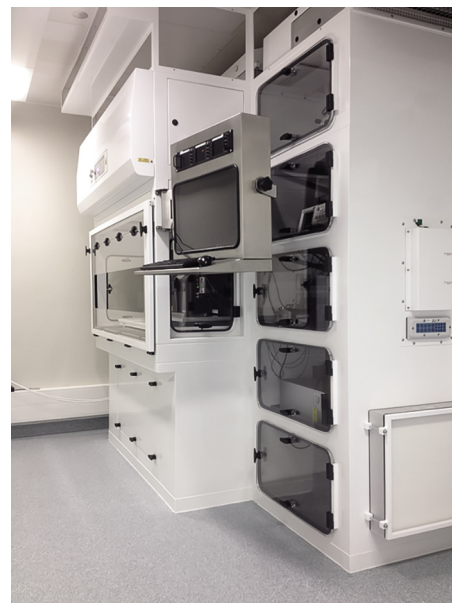
Fig. 3. Droplet sorter for clinical use. GMP-compliant droplet sorter with exchangeable fluidics and accompanying equipment enclosed in a tailor-made laminar air flow bench maintaining grade A. The surrounding room is of grade B. (Photo from Uppsala University Hospital, Sweden)
